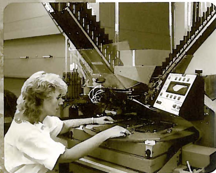
Electronic circuit manufacturing, Bailey Williamsport facility
